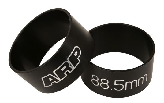
ARP's performance R&D division has just released a new 88.5 MM Piston Ring Compressor tool. ARP Ring Compressors are machined from 6061 T-6 Billet tube material and Type 3 anodized for long life. All ARP Ring Compressors feature a true radius design far superior to conventional "tapered" designs and are relieved for wire O-rings on the bottom. The bore size is prominently engraved in 3/4" high numbers for easy identification.
